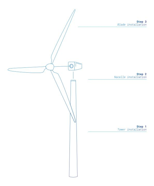
There is talk of using a big DP-HLV in the future for single-lift installation of WTGs, but the technology is not mature and trials have not yet been done for fixed foundation wind farms. However, for floating wind, this has been successfully done.
