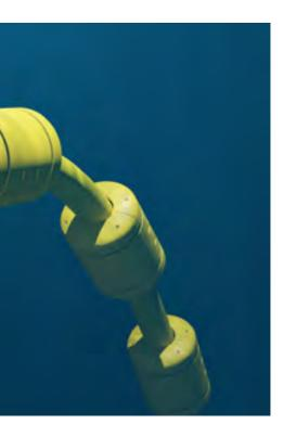
If it's a deep water location, the cables are semi-submersible, designed to be lighter, and floats are attached to them as per the
