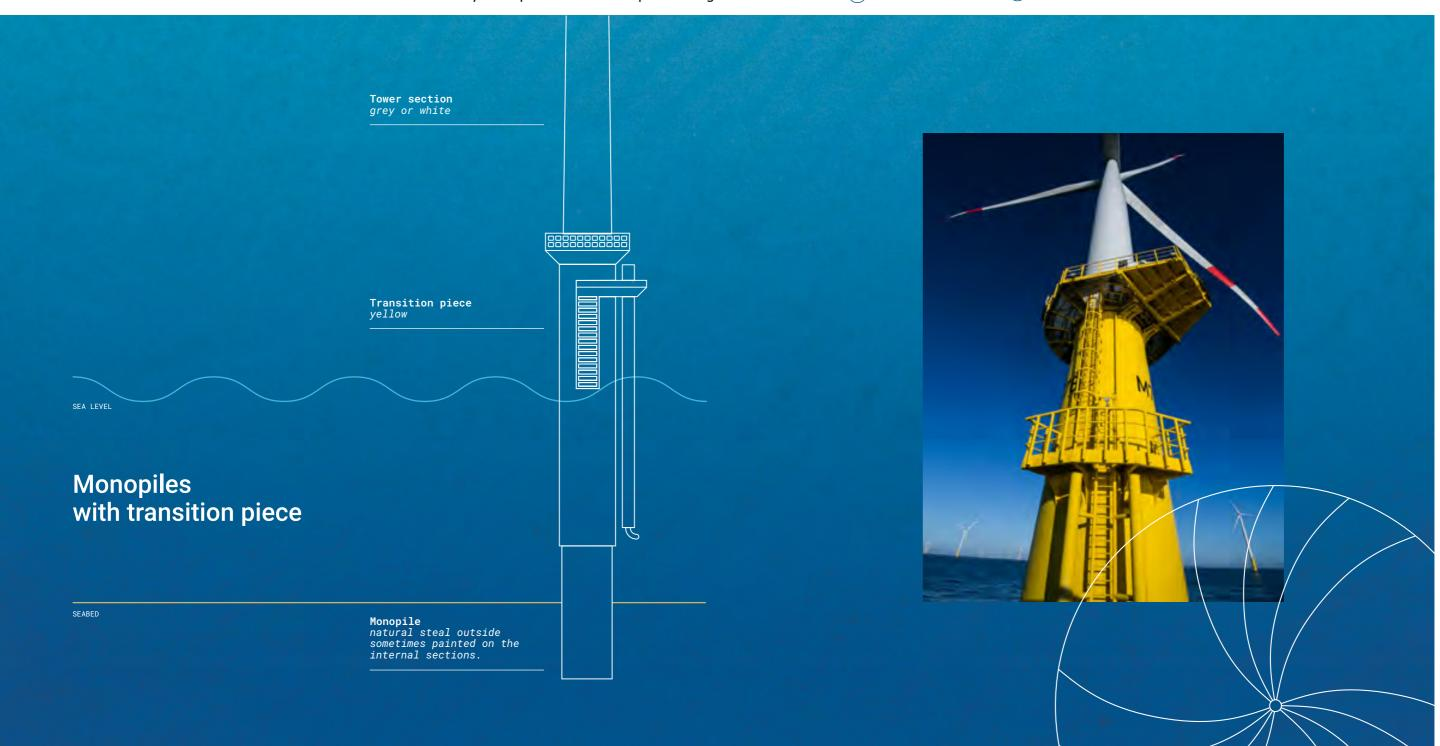
This is the oldest design and is the most commonly used throughout Europe. For this design the monopile will be tapered inwards at the top standing side so that the transition piece can be installed over the pile, with the pile making contact with the internal laydown guides.
